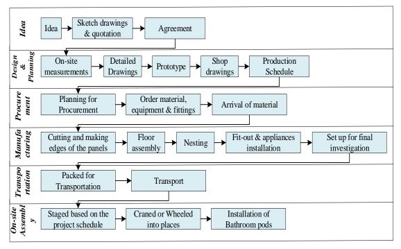
Figure 1: Modular bathroom manufacturing process
