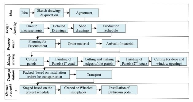
Figure 2: Prefab wall panel manufacturing process
